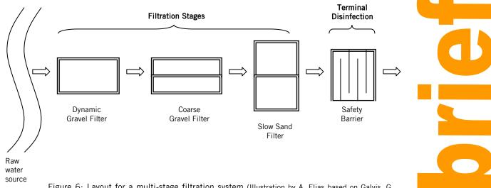
Figure 6: Layout for a multi-stage filtration system (Illustration by A. Elias based on Galvis, G. IRC 2006)
